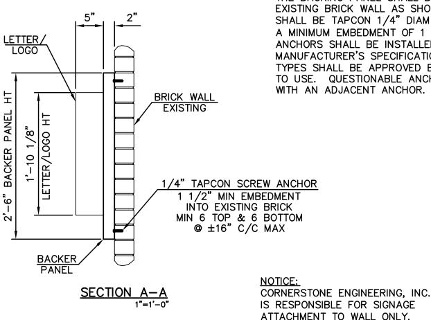
ANCHORAGE NOTE: THE BACKING PANEL SHALL BE ATTACHED TO THE EXISTING BRICK WALL AS SHOWN. THE ANCHORS SHALL BE TAPCON 1/4" DIAM SCREWS ANCHORS WITH A MINIMUM EMBEDMENT OF 1 1/2" INTO THE BRICK. ANCHORS SHALL BE INSTALLED FOLLOWING MANUFACTURER'S SPECIFICATIONS. ALTERNATE ANCHOR TYPES SHALL BE APPROVED BY CORNERSTONE PRIOR TO USE. QUESTIONABLE ANCHORS SHALL BE REPLACED WITH AN ADJACENT ANCHOR.
